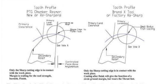
The Flute face is the Work Horse. As the coated flute face plunges in to the cavity it lifts and seperates the material (Chip Removal). That is the reason that cutting tools with burnish wear bar "margin" can be circle ground after coat, as it only burnish the Reamed circumfrence. This gives a Great Finish with Long Life.
